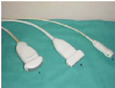
Curved (A), linear (B), and sector (C) array transducers provide differing shapes in the ultrasound field-of-view.
